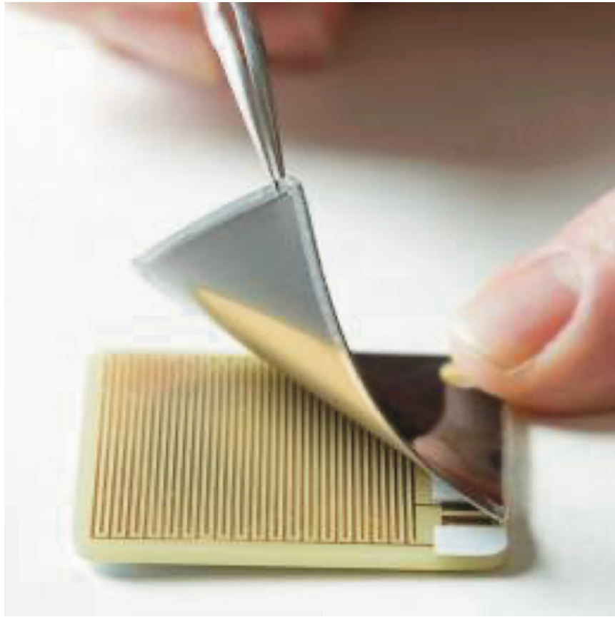
Above: Adhering XactFSR over copper conductors. Note the narrow border of adhesive at the edge of the XactFSR.
